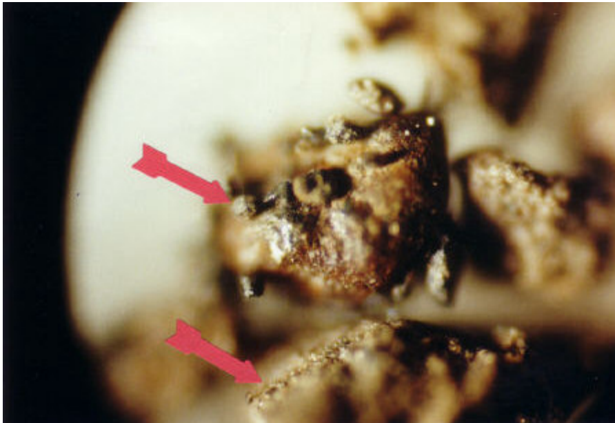
Fig. 11: Photomicrograph (x 100) of Magnetic Material--Both Spherical and Partially Ablated--Adhering to Soil Chunks (KS-04-176). [Note melted ridge of magnetic material at lower arrow.]
